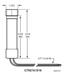
The Solid State Ultraviolet Flame Detectors detect the ultraviolet radiation emitted by combustion flames. The flame detectors are used with Honeywell flame safeguard controls to provide flame supervision for gas, oil, or combination gas-oil burners.
